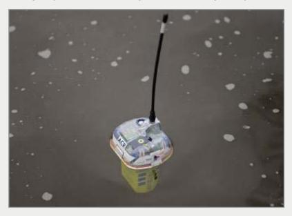
These floating radio distress beacons can transmit for hours. They can be manually activated or can float free from a sinking or overturned vessel. Their signals give your position to a network of satellites, which then sends it to Joint Rescue Coordination Centres. They play an important role in an emergency. Although pleasure craft are not required to carry them, they are a very good idea.
