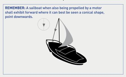
Read the <u>Collision Regulations</u> (referred to in each of the following categories) for more details. **If you are fitting your own navigation lights**, refer to the positioning requirements in the <u>Collision Regulations</u> (ANNEX I: Positioning and Technical Details of Lights and Shapes).
