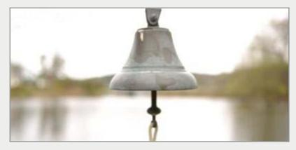
All boats 12 m (39'4") or more must have a fitted whistle. Boats over 20 m (65'7") must also have a bell. Check Annex III of the <u>Collision Regulations</u> for the technical standards these appliances must meet.
