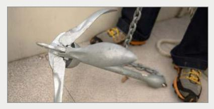
Having the right anchor and cable (refer to SAFETY EQUIPMENT REQUIREMENTS section) for your boat is important. If you do not, rough winds and water can cause it to drag, leaving your boat to drift. This is especially dangerous if you are asleep or swimming nearby. Make sure your boat is well anchored and keep watch to detect signs of dragging.
