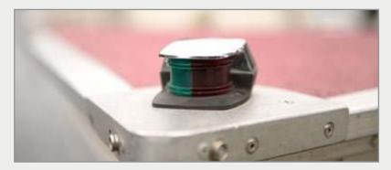
Navigation lights help prevent collisions by making your vessel and its direction of travel more visible to others. Vessels near you will make decisions based on the information your lights provide. The navigation lights on other vessels can help you tell the direction they are moving or whether they are at anchor or engaged in some other activity.
