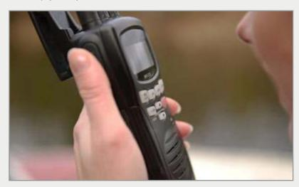
Marine VHF radio is generally the best way to send a distress alert. If you have a VHF radio, keep it tuned to channel 16. Know where you are at all times and be prepared to describe your specific location.
