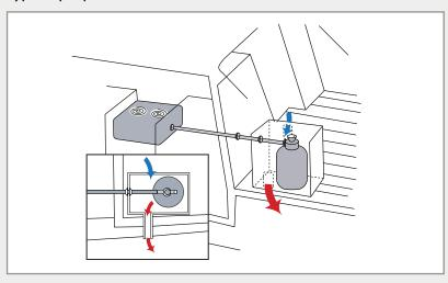
Gas vapours and leaking propane and butane are heavier than air and will quickly flow into the lower parts of your boat. They are very hard to remove and are **highly explosive**. On board appliances that run on propane or butane may present more risk than gasoline.
